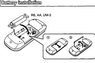
Insert the batteries observing the correct polarities  $(\oplus, \Theta)$ .
